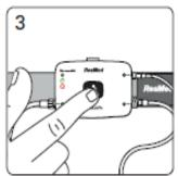
Press and hold the power button for about three seconds to turn off the device.
