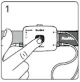
Press and hold the power button in the centre of the device for about three seconds or until the light turns on.
