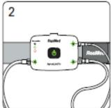
Check that lights next to the accessories you are using are green. If any of these lights are red and blinking, the accessories are not attached correctly.
